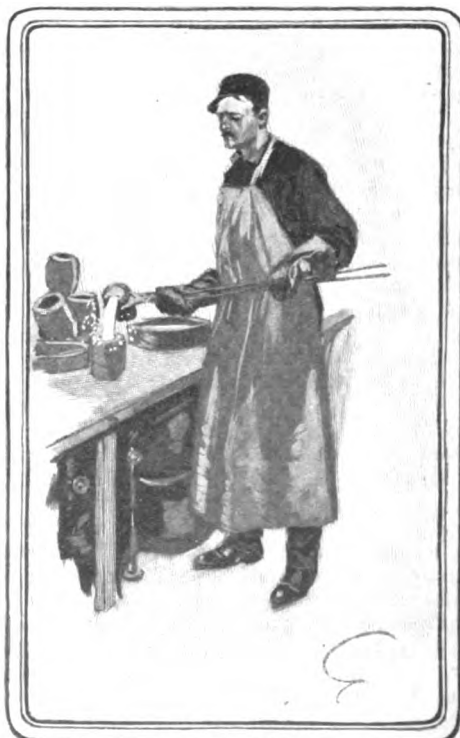
IN THE ASSAY OFFICE—POURING MOLTEN GOLD FROM THE CRUCIBLE INTO THE MOLDS THAT FORM IT INTO BARS WORTH ABOUT EIGHT THOUSAND DOLLARS A PIECE.
